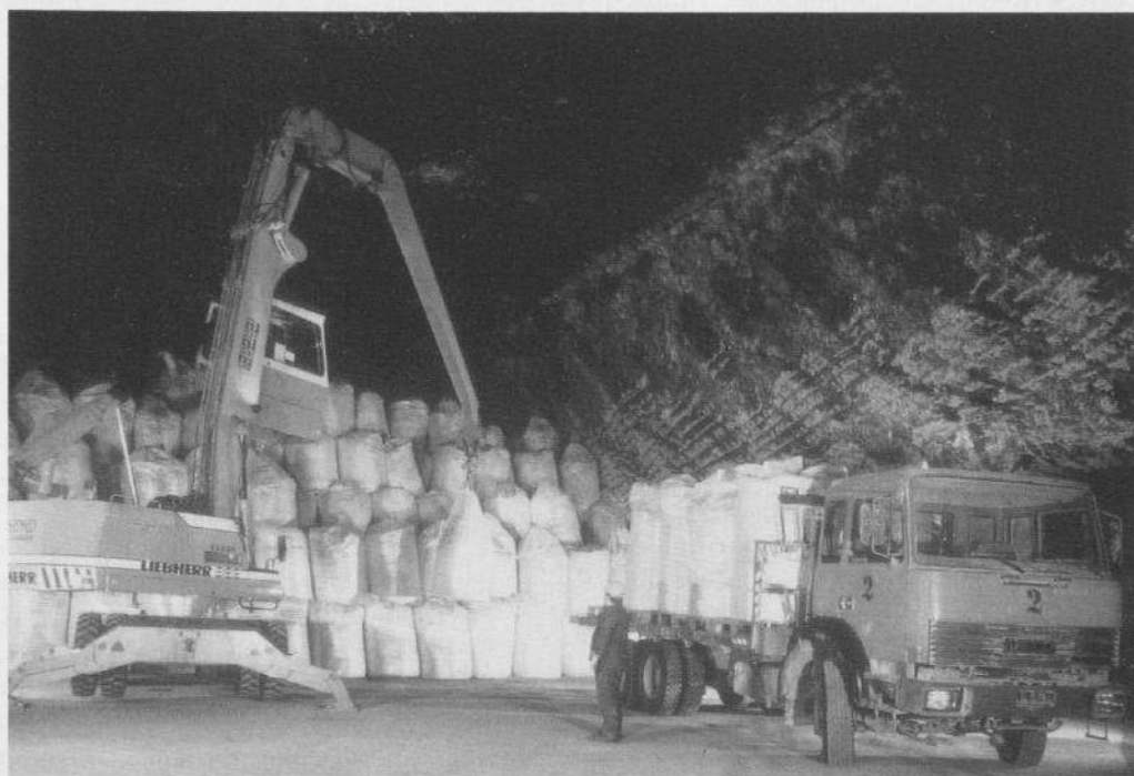
Fig. 7: Stacking of big bags by a mobile crane
